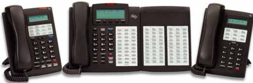
ESI desktop phone models, left to right: 24-Key Digital Feature Phone, 48-Key Digital Feature Phone with optional 60-Key Expansion Console, 12-Key Digital Feature Phone.
